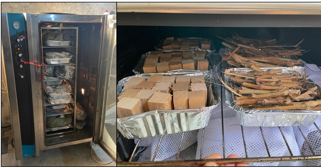
Figure 9. Drying organic materials in the oven at 60° C following their retrieval from the sea
